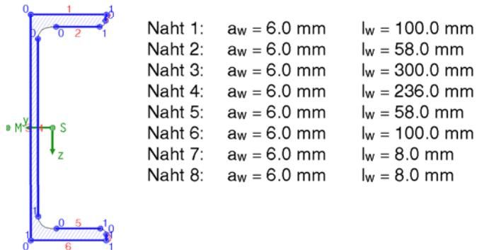
Max:  $\sigma_{1,w,Ed} = 421.53 \text{ N/mm}^2 < f_{1w,d} = 435.56 \text{ N/mm}^2$ ,
