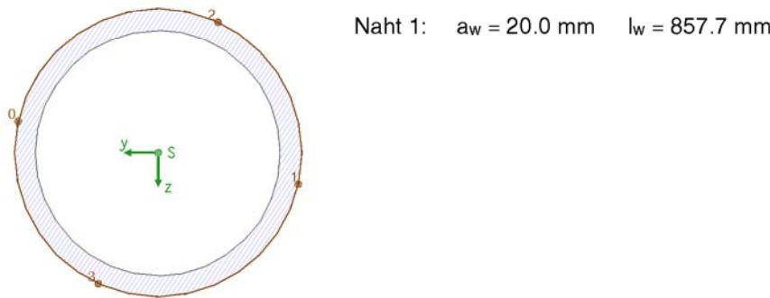
Max:  $\sigma_{1,w,Ed} = 174.15 \text{ N/mm}^2 < f_{1w,d} = 435.56 \text{ N/mm}^2$
